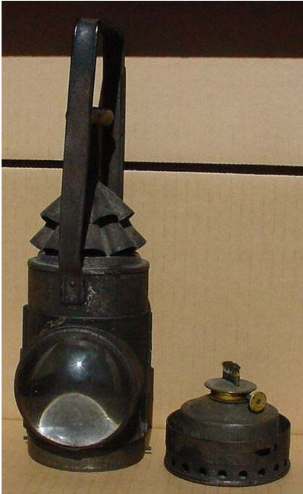
Fuel container and wick from the early lantern. This container is essentially unscrewed from the lantern base.
