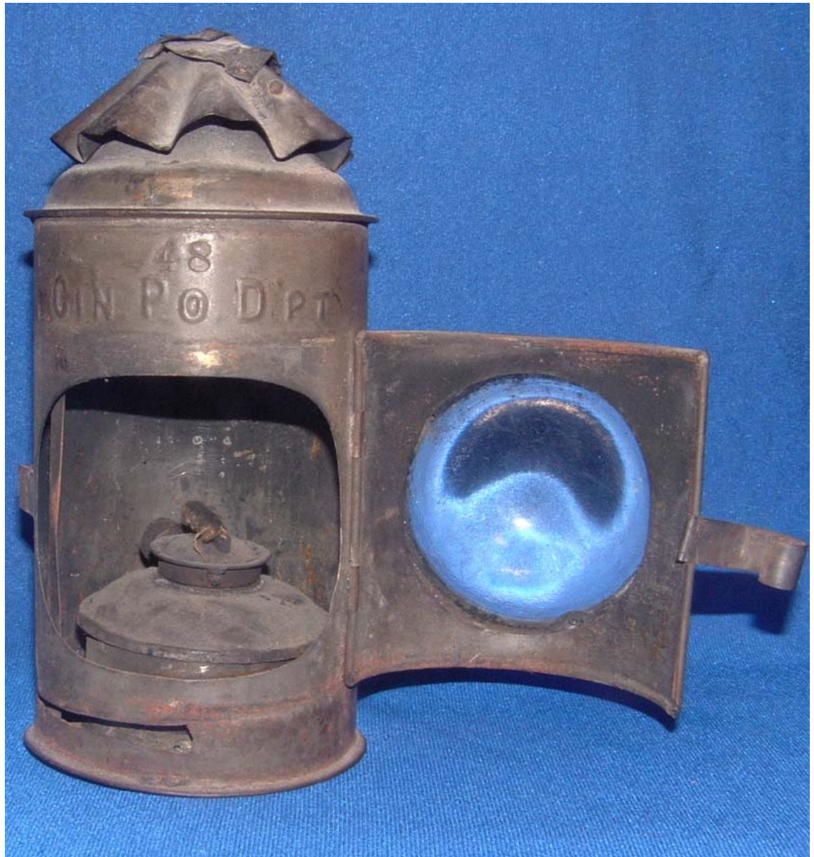
The second style lantern showing the inside where the fuel container sits. The fuel container can be lifted out.
